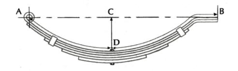
Step 1. Measure along the edge of the top leaf following its curve from A to the centre of bolt hole D
