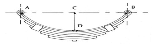
Step 1. Measure along the edge of the top leaf following its curve from A to the centre of bolt hole D Step 2. Repeat step 1, this time from B to the centre of bolt hole D Step 3. Measure the camber or C to D 1. Measurement of Leaf A-D 2. Measurement of Leaf B-D 3. Camber of Spring C to D 4. Width of Spring 5. Number of Leaves 6. Leaf Thickness 7. Diameter of Shackle Pins 8. Greaser Pins? ☐ Yes ☐ No 9. Front or Rear Spring? (For tandem only) ☐ Front Rear 10. Diameter of Centre Bolt
